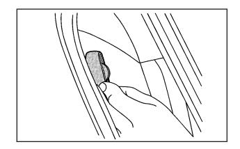
Pull the elastic cord out from between the edge of the seatback and the interior body to remove the guide from its storage clip.
